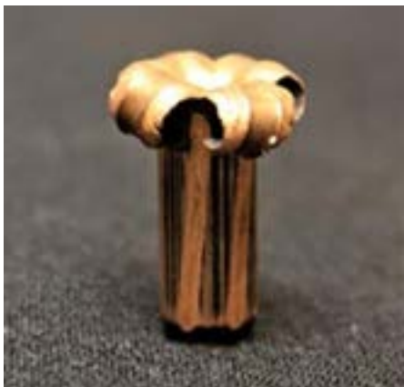
Close-up of an expanded E-Tip retaining 95 per cent of its original weight.
